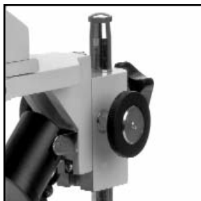
Post-arm design for increased working distance
